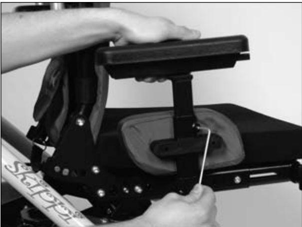
Setting the height of the side panel
