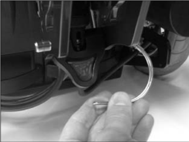
Folding the securing bow
