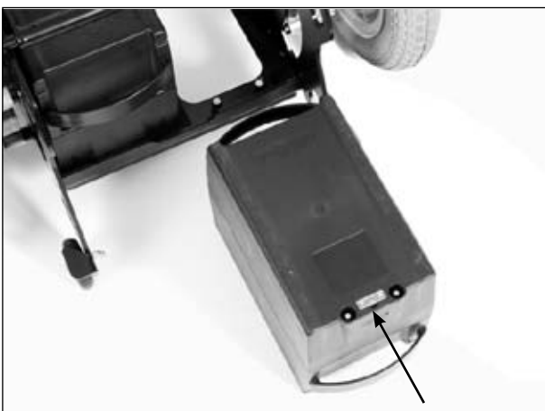
Battery pack with fuse
