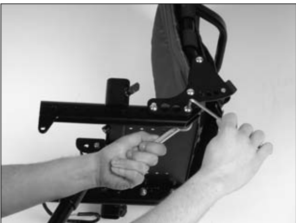
Loosening the bearing plate
