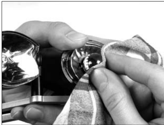
Figure 34 Replacing the front direction indicator lamp
