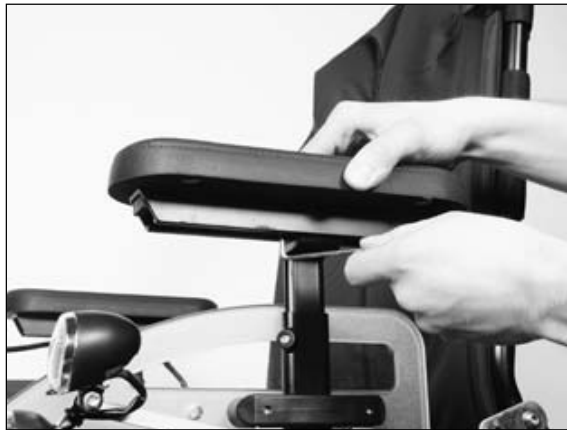
Figure 57 Adapting the arm rests to the forearm length
