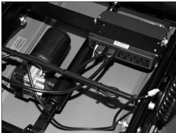
Figure 71 Seat bracket position for the seat tilt unit (example) and actuator connection on the seat module
