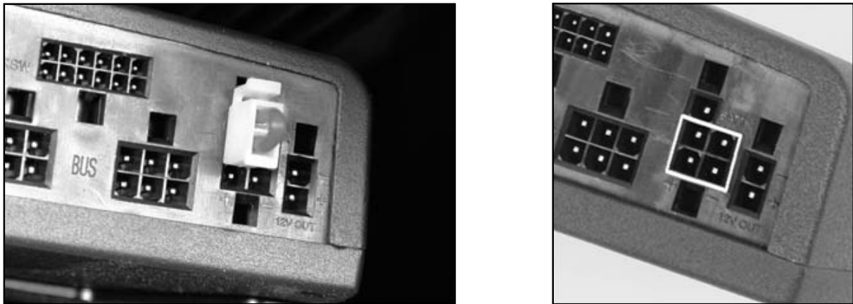
Figure 112 Battery connection for power supply
