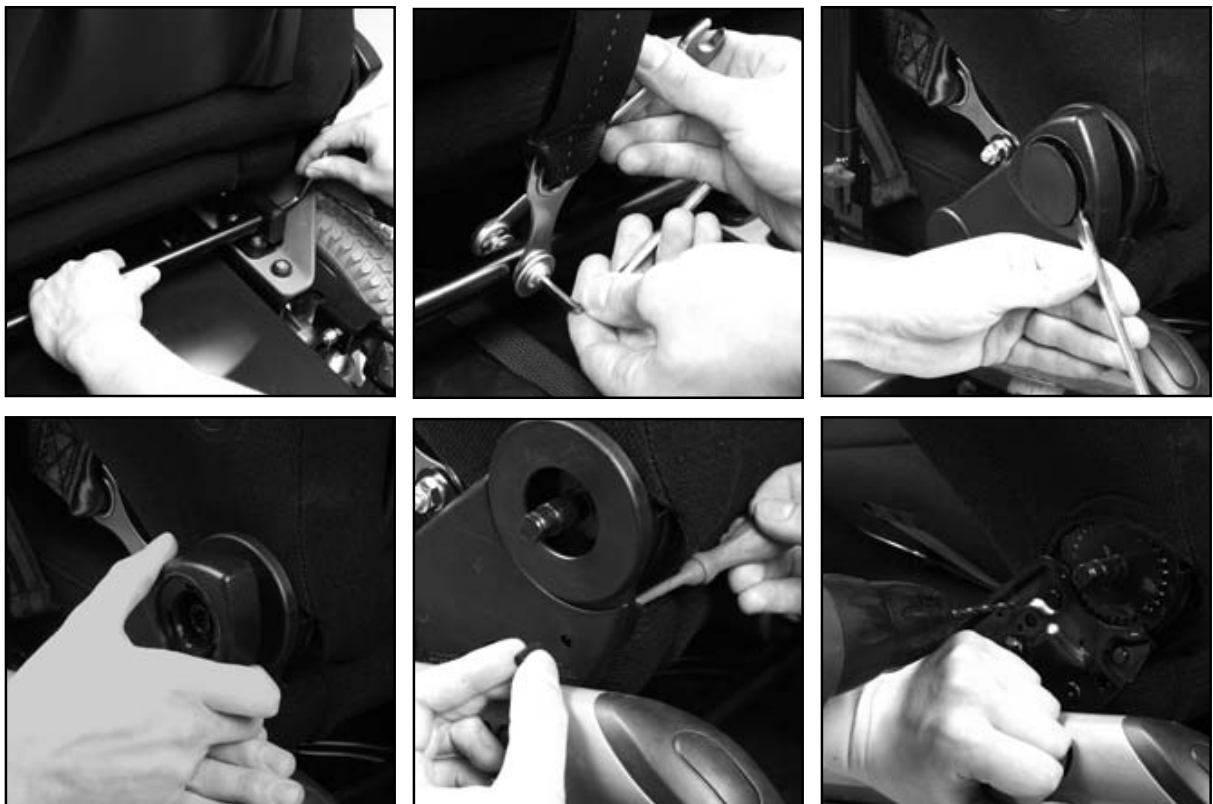
Figure 60 Installing / retrofitting the four-way chest strap
