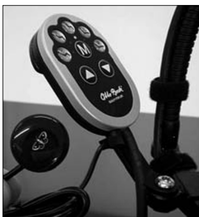
Figure 102 Connecting an external switch (here: Buddy Button) to the push button module
