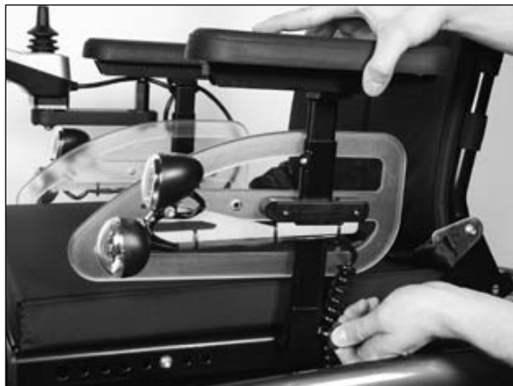
Figure 55 Loosening the thumb screw for removal of the side panel with arm rest
