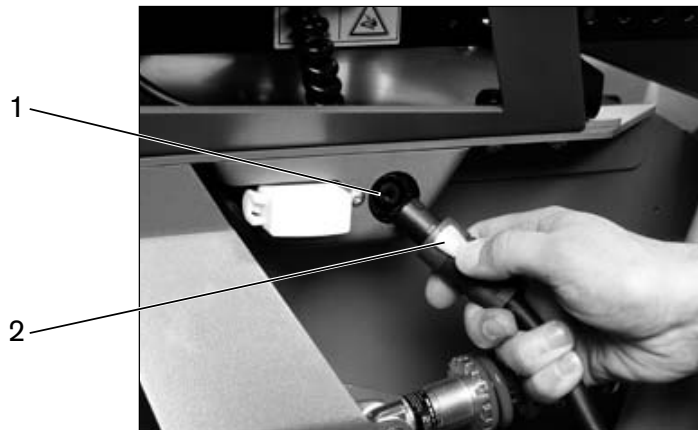
Figure 9 Connecting the charger to the charging receptacle
